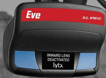
**“STARTS RECORDING WHEN TRIGGERED BY FOLLOWING TOO CLOSELY, A HARD BRAKE, SPEEDING, ROLL STABILITY, OR LANE DEPARTURE, THE CAMERA CAPTURES 12 SECONDS OF VIDEO.”**
